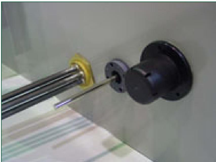
Our factory-installed heaters keep the water temperature at 4°C and act as a simple and economical **anti-freeze measure for the basin water**. The heater package includes the **heaters**, a **thermostat** and a **low level cut out switch** to protect the heaters if the water level declines excessively. Standard electric heaters can handle ambient temperatures down to -18°C.
